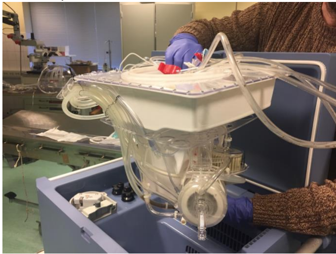
Disposable parts of heart perfusion system developed by Prof Stig Steen
